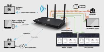
The Dual-Cam function allows you to offer different perspectives to remote online participants by using two USB cameras alternately for BYOM meetings wirelessly on your laptop or, thanks to the Dual-UCC function, also via USB cable on a stationary room PC.
